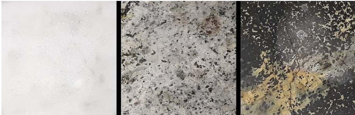
Figure 4. Photograph of the three tested rocks: marble ( left ), copper ore ( center ), and nickel ore ( right ). The dimensions of sample imaged are about 50\text{ mm} \times 50\text{ mm} . Marble has a high degree of homogeneity, while ores show random inhomogeneities in size and distribution.
