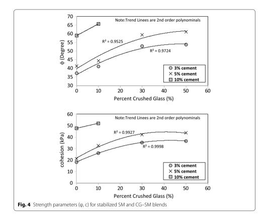
stabilized SP increased significantly as the percentage of CG increased. Considering that CG aggregates have sharp corners, by addition of CG, fastening between aggregates grew up, and the adhesion between the aggregates may also increase the shear resistance.
