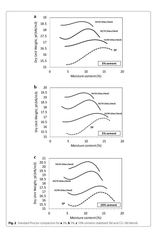
For example, increasing in the amount of cement from 3 to 10% could contribute to increase in the sandy soil  $\gamma_{d,max}$  from 16.6 to 18.71 kN/m<sup>3</sup> (about 3%). While this proportion of cement, Addition of the crushed glass in mixed 50% CG–SP will increase amount  $\gamma_{d,max}$  from 18.71 to 20.66 kN/m<sup>3</sup> (approximately 11%).Therefore, (as shown in Fig. 3) the values of  $\gamma_{d,max}$  increased in a nearly linear fashion with CG increment, which
