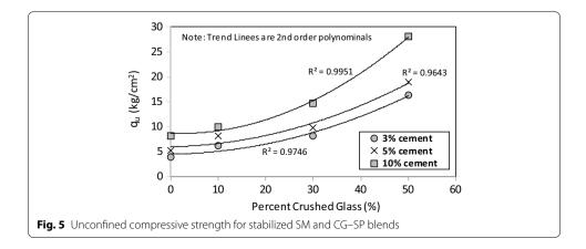
due to the replacement of cement with sand grains and increasing pozzolanic reactions between grains.
