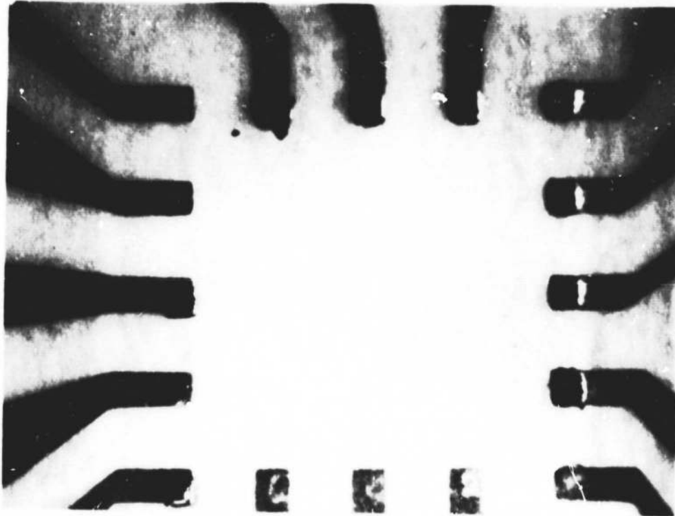
THIN FILM Mo/Au SUBSTRATE METALLIZATION AFTER DEVICE SHEAR TESTS
