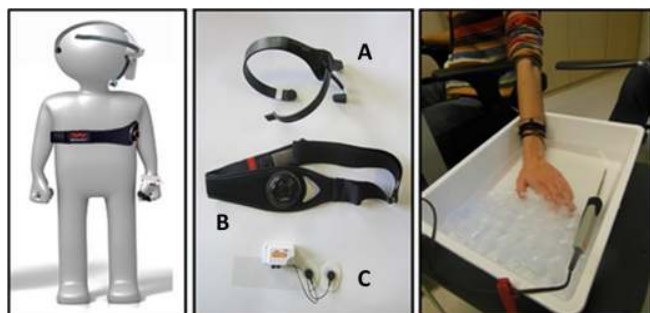
Fig. 1. Left and centre panels: Wearable sensors used to acquire physiological signals and their specific way to be worn; A) MindWave Mobile EEG headset, B) Zephyr BioHarness™3 (BH3) chest belt, C) Shimmer Sensor. Right panel: Picture depicting the execution of the cold pressure test.
