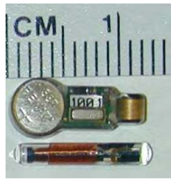
Figure 2.1. The ATS JSATS Acoustic Micro-Transmitter (Top) and a PIT Tag (Bottom)
