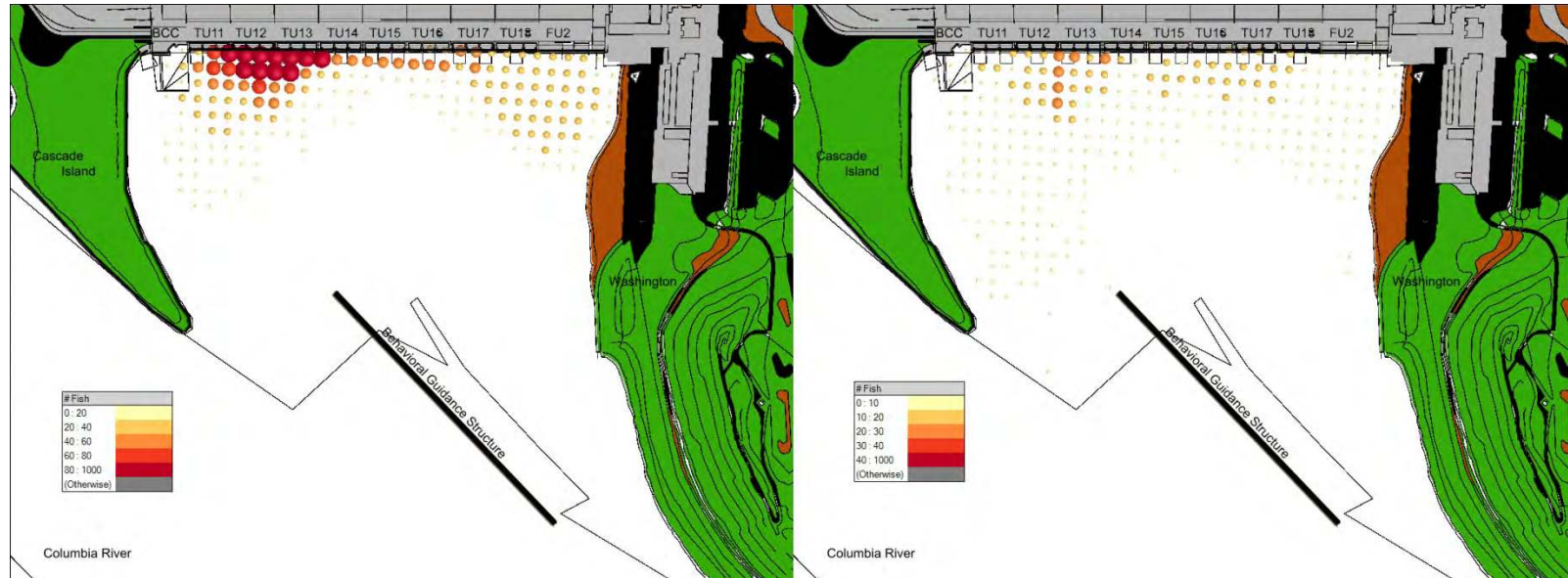
Figure 3.18. Total Number of Fish Tracked Within 10-m x 10-m Grids During Daytime (Left) and Nighttime (Right) and for Yearling Chinook Salmon Smolts Approaching B2. Sphere size and color are a function of the number of fish in detected in each grid for all of the springtime period, and individual fish are only counted once per grid. Grids without tracked fish are not displayed; however the entire B2 forebay was included in this analysis.
