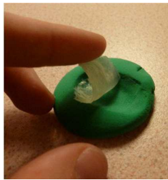
Figure 6. A prosthetic finger created out of latex at the GREYC research laboratory.
