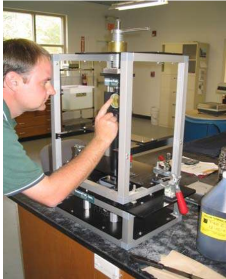
Figure 9. ATACKER™ Device for Tack Coat Bond Strength
