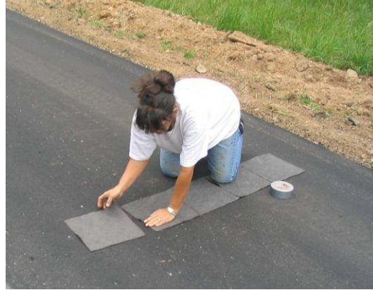
Figure 20. Placing Pads for ASTM D 2995
