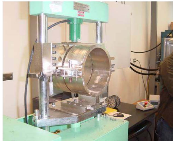
Figure 7. FDOT Bond Strength Device
