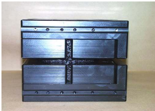
Figure 5. Shear Box with Prepared Sample
