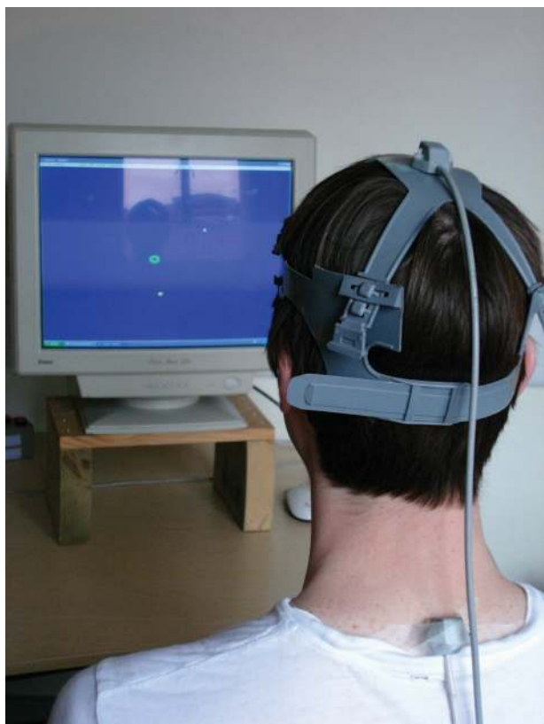
Figure 1. Experimental setup for the head-tracking cervicocephalic kinesthesia test. The distance from the head-mounted sensor to the screen center is 80 cm. The yellow cursor provides the visual target, and the green, ring-shaped cursor displays head position.
