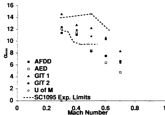
Figure 7. Comparison of angle of attack for the maximum lift coefficient with Mach number.
