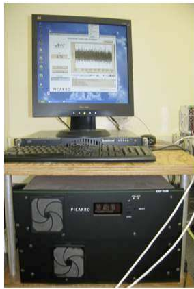
Figure 4. Instrumentation. a) Picarro CRDS EnviroSense NH 3 analyzer; b) SS bubbler and parallel flow controllers for testing of 4 tubes simultaneously.
