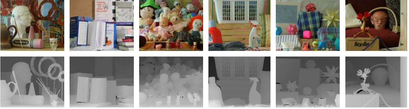
Figure 3. The new Art, Books, Dolls, Laundry, Moebius, and Reindeer stereo test images with ground truth.
