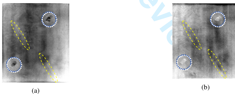
Figure 9. First time derivative image (left) at t=2.6 s and second time derivative image (right) at 5.2 s in the 150 s heating procedure and working on the frame rate of 30 Hz.
