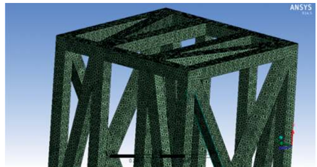
FIGURE 4: Mesh elements for the test rig analysis.
