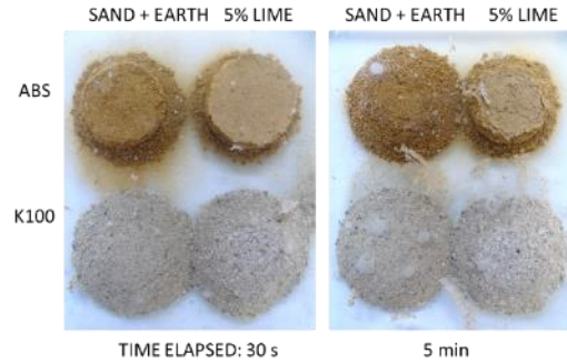
Fig. 11 Submersion test, the second column in each picture is with the lime addition.
