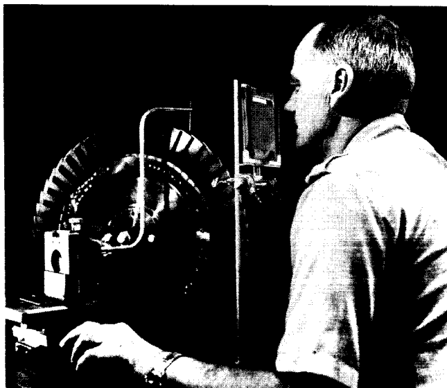
Figure 9.—Imaging and viewing a localized interference-fringe pattern.
