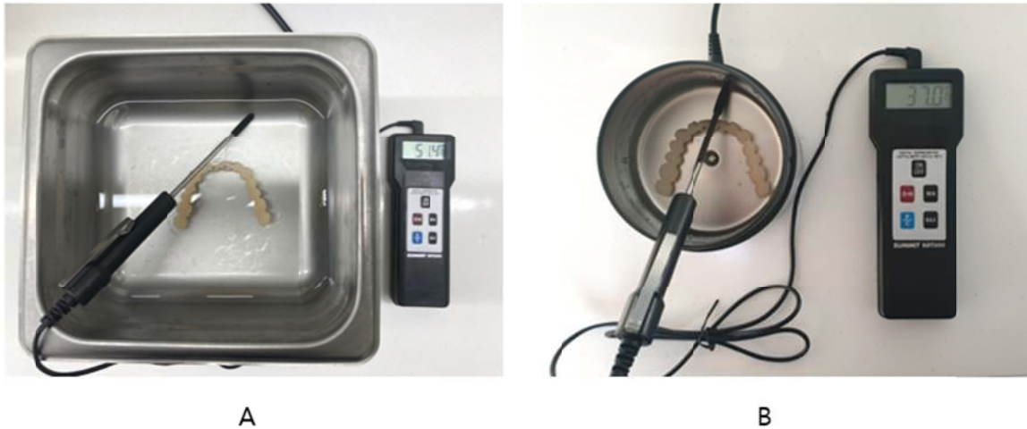
Figure 5. Ultrasonic cleaning of full arch artificial teeth and digital temperature measurement. (A) General ultrasonic cleaning, (B) ultraviolet-C ultrasonic cleaning.
