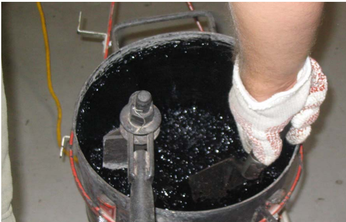
Figure 5. Warm Mix Asphalt in Bucket Mixer.
