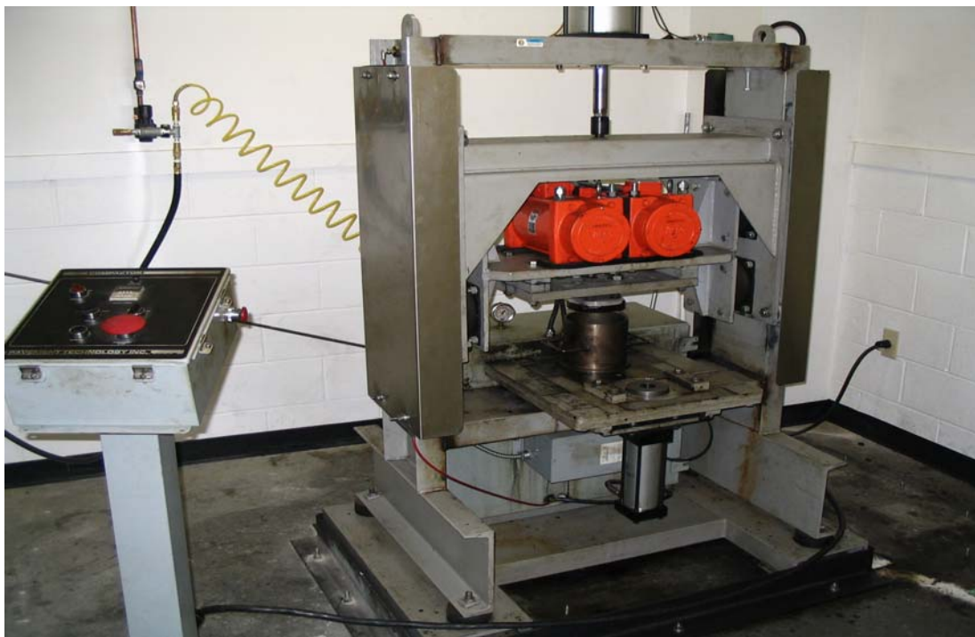
Figure 2. Vibratory Compactor used for Compaction of Test Samples.
