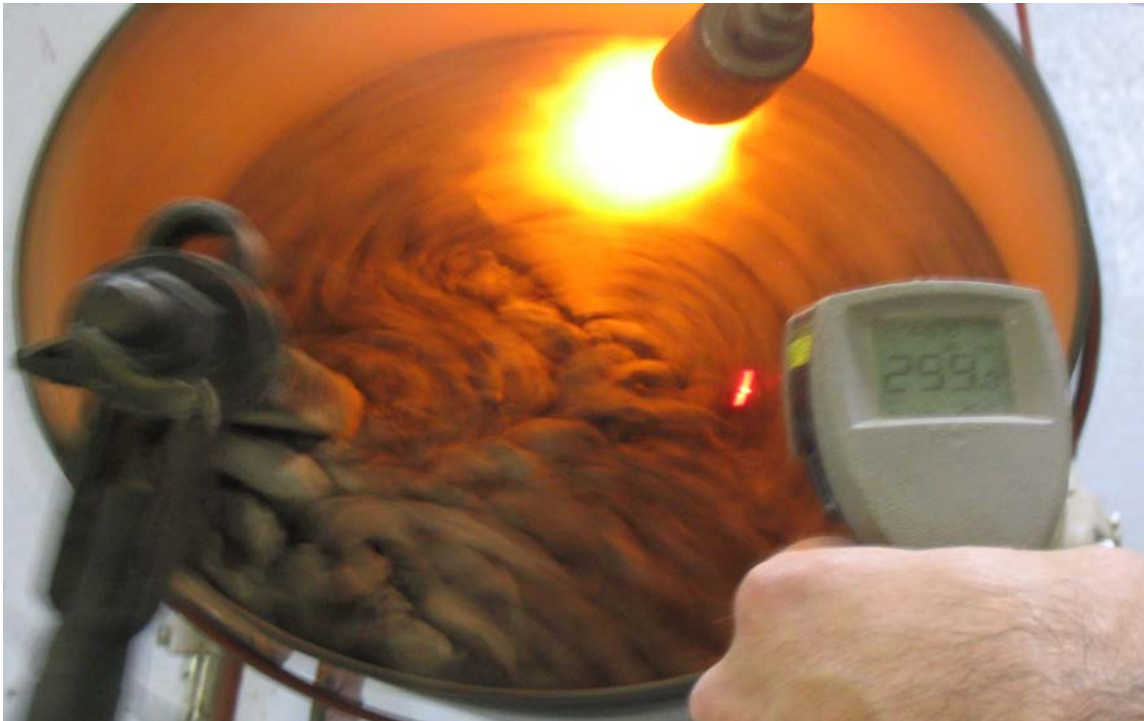
Figure 4. Heating of Wet Aggregate to Mixing Temperature.
