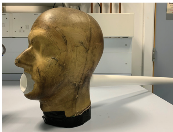
Figure 4. Cough simulator cough delivery point attached to the 'wearer' manikin head.
