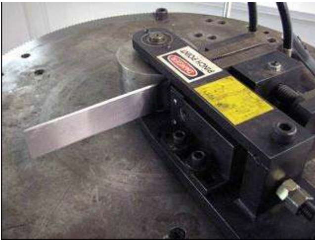
Figure 11 (left). Bend specimen before test.
