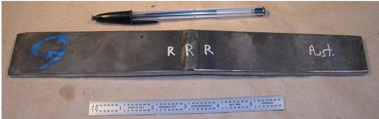
Figure 3. Location of three residual stress and one retained austenite measurements on top of the plate.
