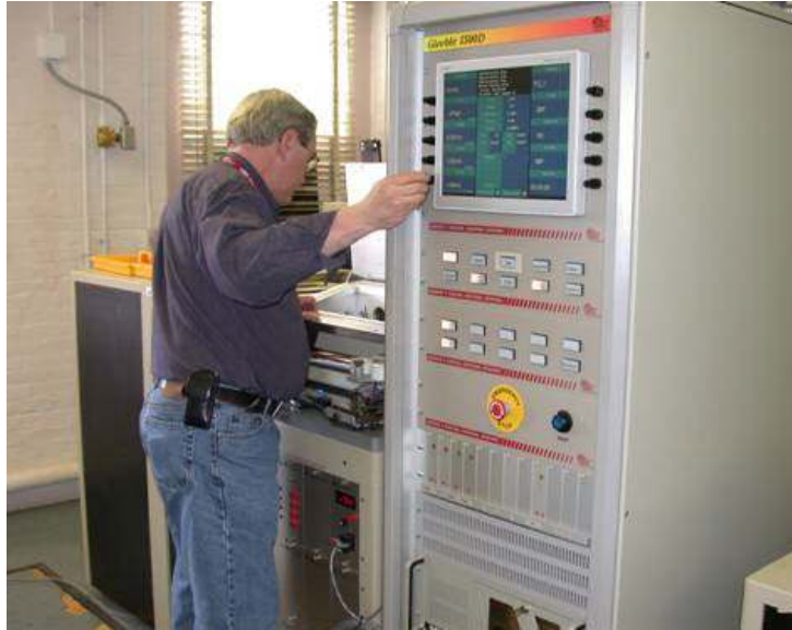
Figure 5. Gleeble 1500 at Benét Laboratories used for HAZ simulation testing.
