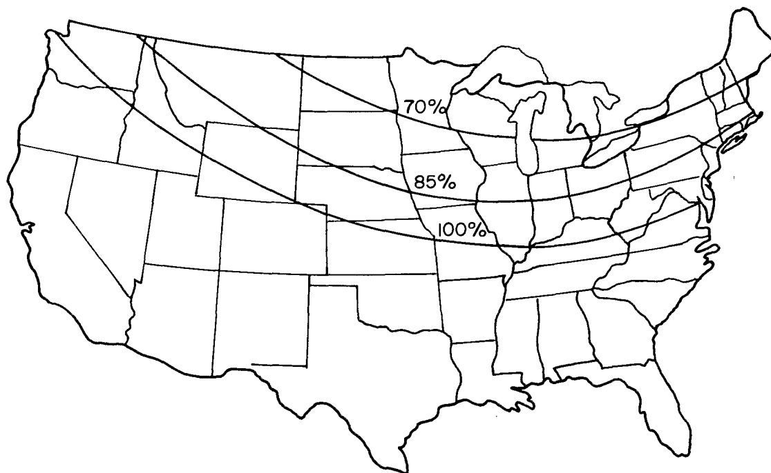
Figure 21. Contours of the conventional gas or oil furnace efficiency required to save more primary energy than the best alternative system (from Ref. (57)).
