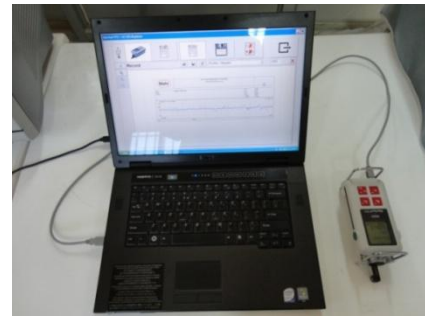
Figure 2. Mahr-PS1 surface roughness measuring unit
