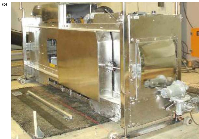
Figure 8. One-third scale MMLS3: (a) schematic, units in mm and (b) MMLS3 mounted on top of a laboratory pavement slab.
