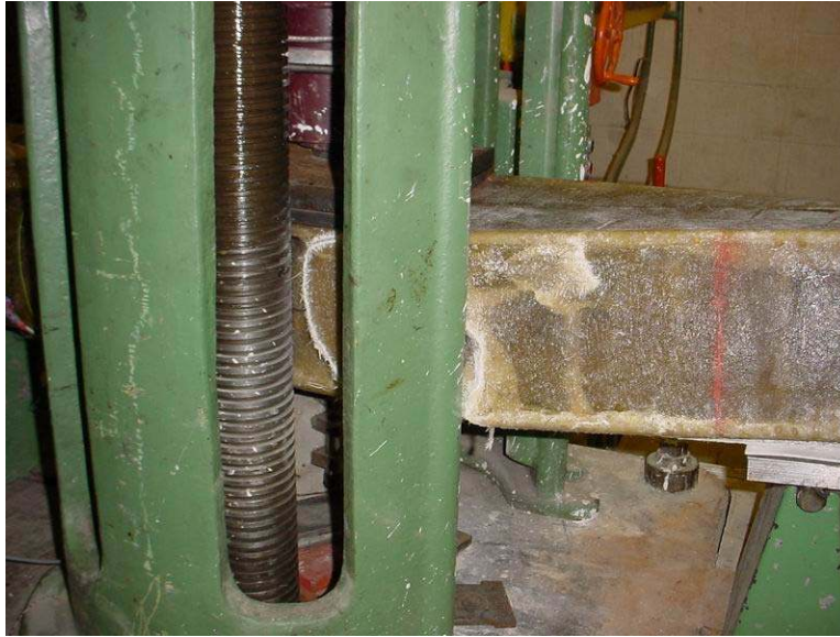
Figure 5-16 Failure mode in Test 1 – side view
