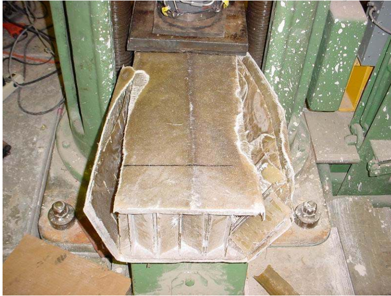
Figure 5-29 Buckling of the core in Test 2
