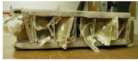
Test 4 – 0.5-in.-thick faces
