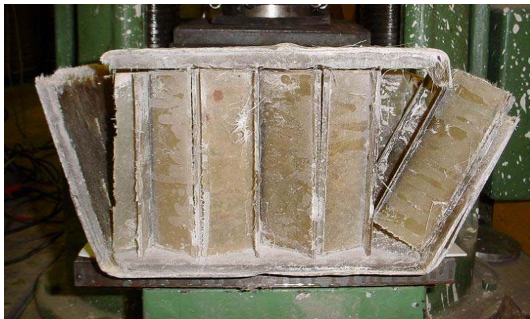
Figure 5-28 Debonding at top face-core interface in Test 2
