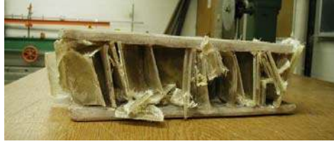
Test 1 – 0.375-in.-thick faces
