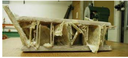
Test 2 – 0.375-in.-thick faces
