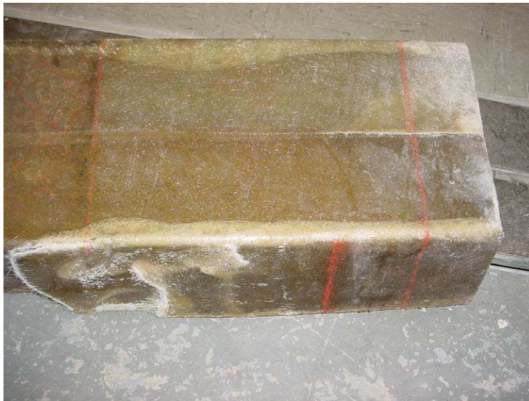
Figure 5-17 Local buckling of the core in Test 1
