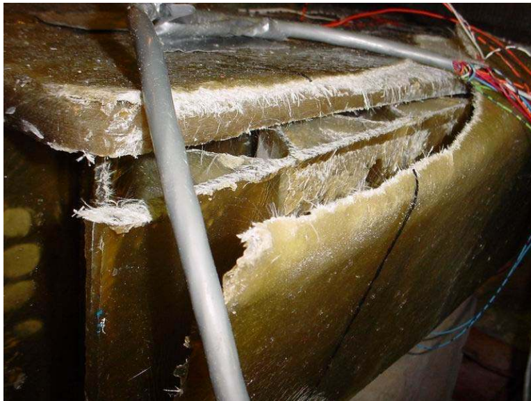
Figure 5-45 Debonding at the face-core interface in Test 4
