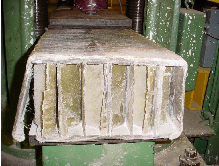
Figure 5-18 Failure mode in Test 1 – end view
