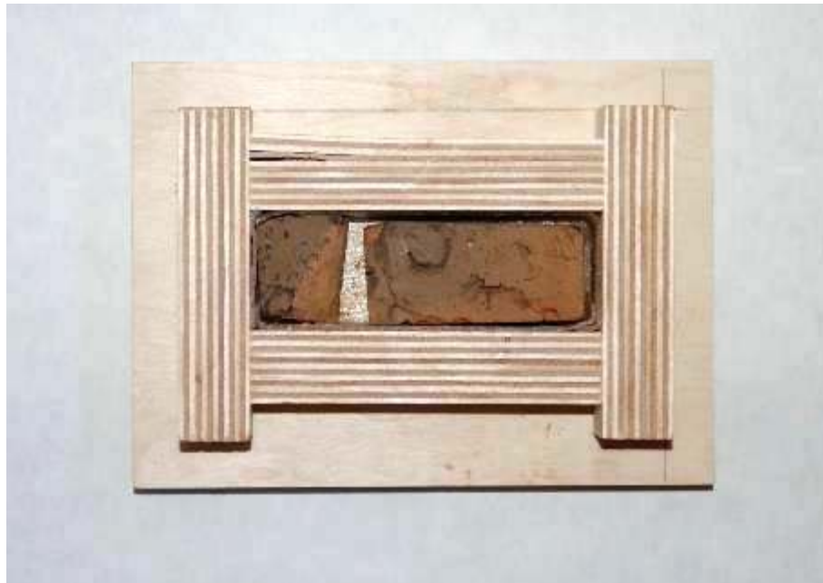
Figure 6.7: View of the prism to be injected at a distance of 5 mm
