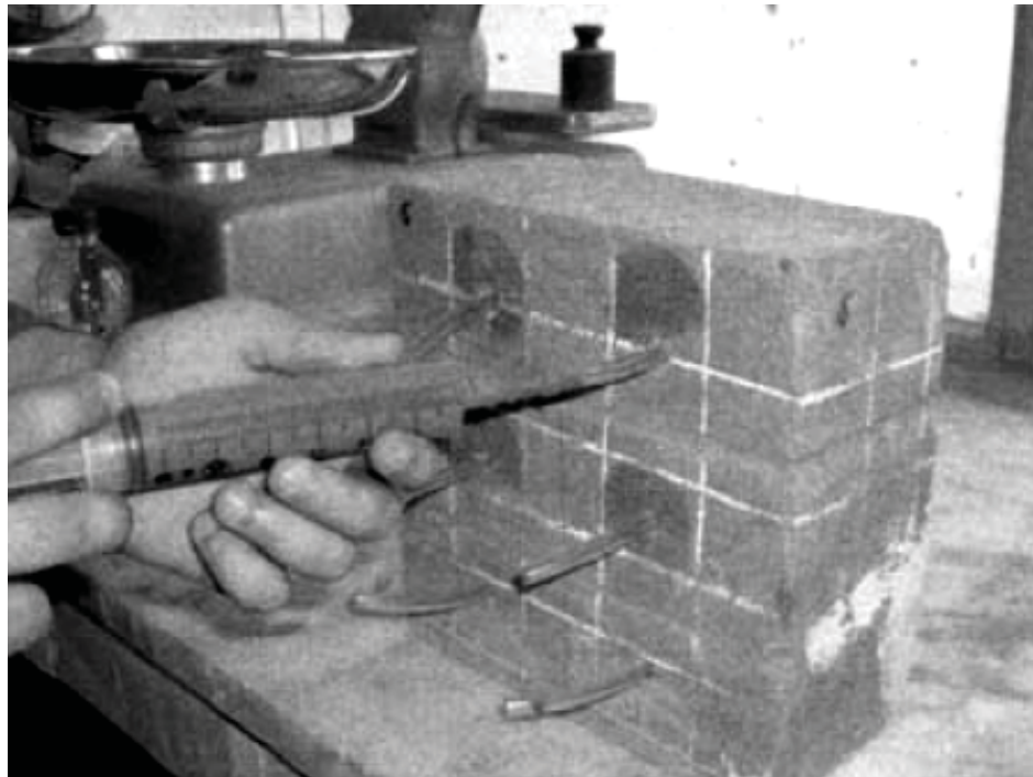
Figure 10.3: View of Clay-Lime-Pozzolan bars to create stronger zones in Masonry. (Vintzileou. E, 2006)
