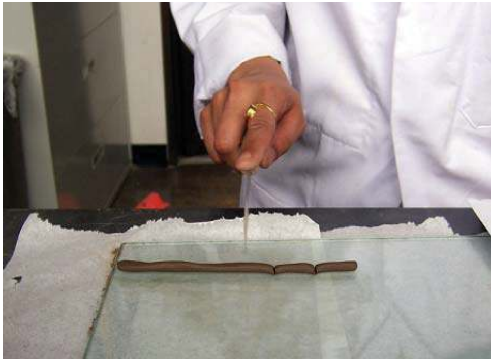
Figure 6.10: Cutting the 3 mm ellipsoidal hand rolled soil into six halves
