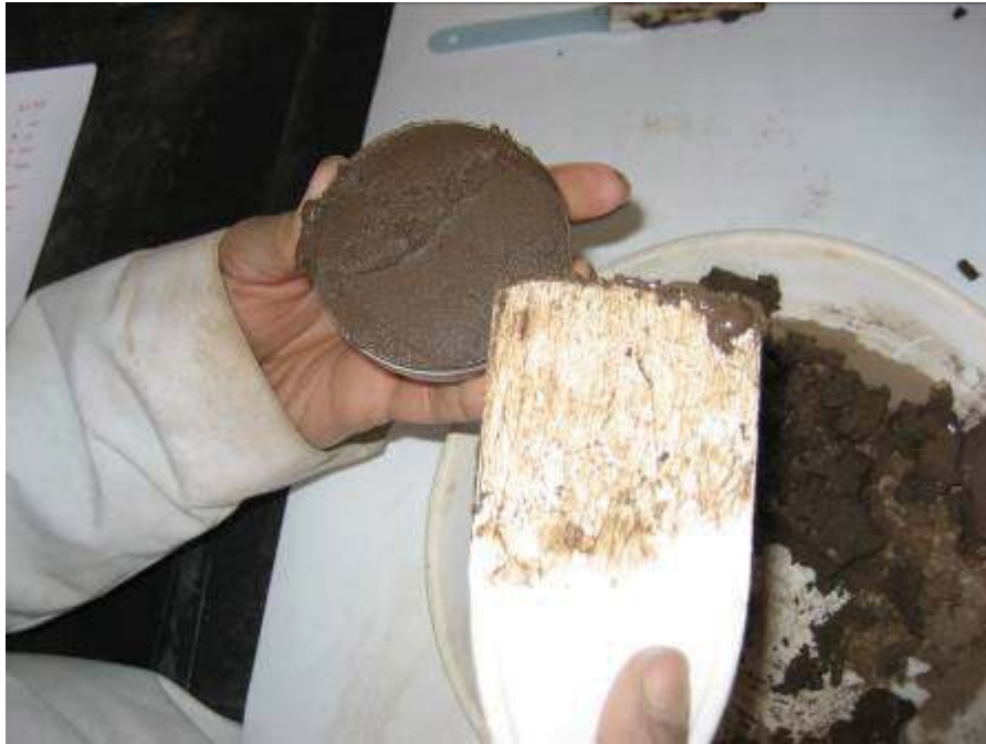
Figure 6.12: Casting the wet soil into shrinkage dishes
