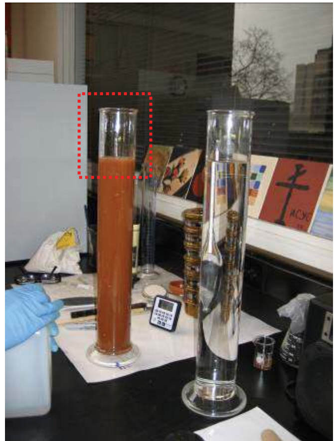
Figure 6.9: Sedimentation of Fine Particles in 1000 ml cylinders
