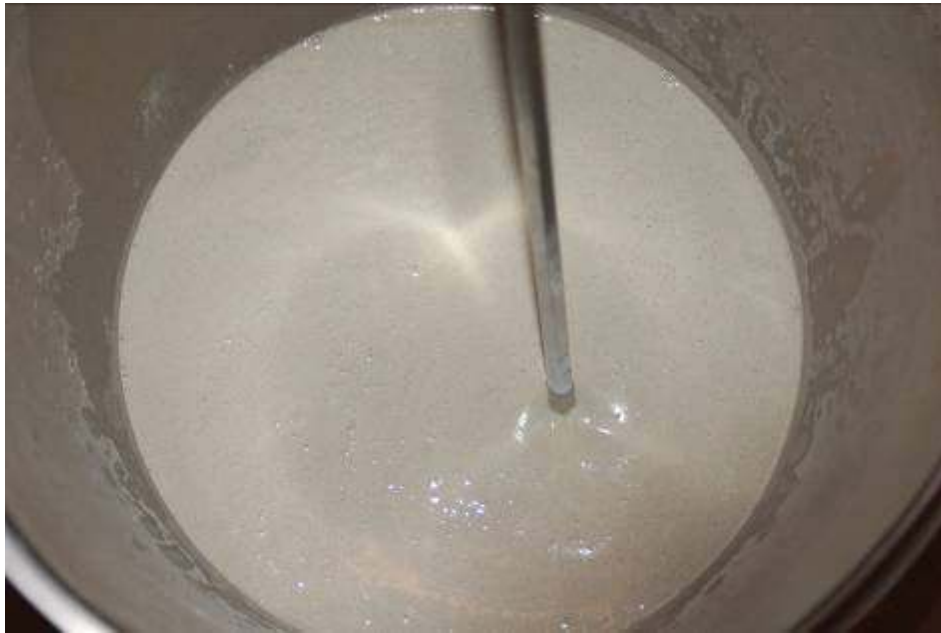
Figure 6.5: High turbulence mixing with Milwaukee drill
