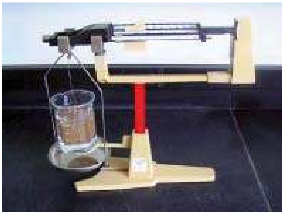
Figure 6.15: Triple beam Balance for hydrostatic weighing of samples
