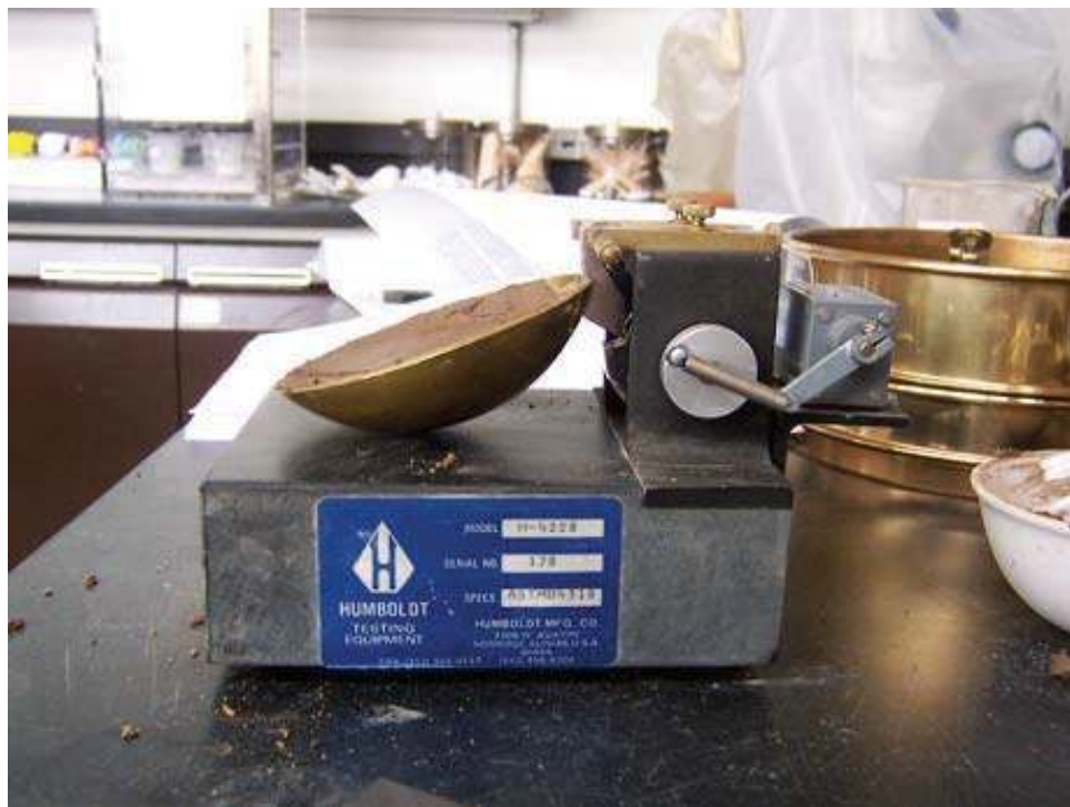
Figure 6.11: Casa Grande Device for Liquid Limit calculation
