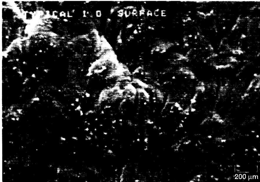
Figure 16.—Typical carbon deposit in 304 SS tube. Granular structure indicating progressive nucleation and growth.
