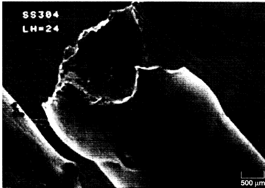
Figure 12.—Initial test failure showing pinholes and significant plastic deformation (304 SS).
