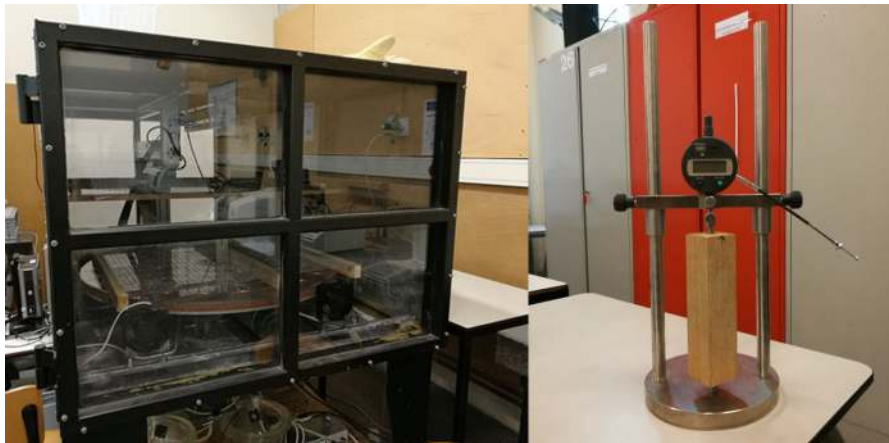
Fig. 3 Setup of the drying shrinkage test: constant humidity curing and measuring
