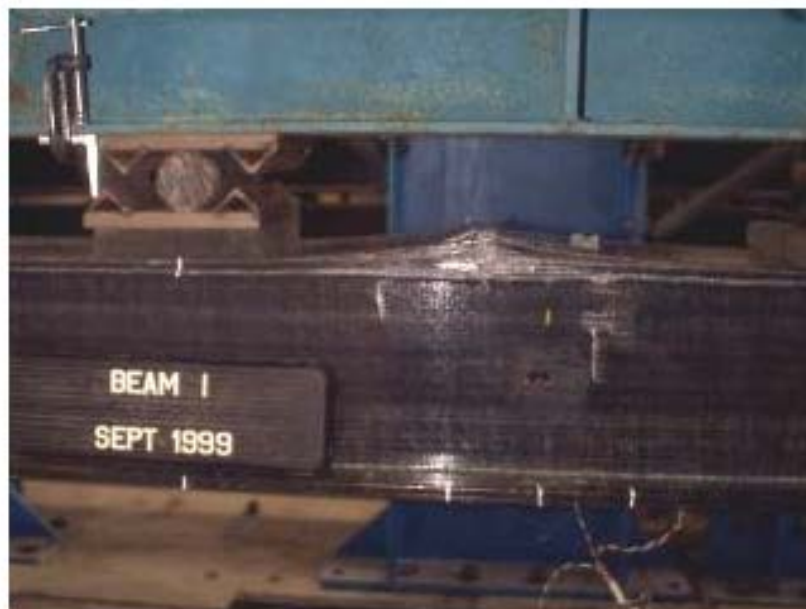
Figure 8. Failure of the compression flange for removed Tom's Creek Bridge FRP composite Girder 1. Note failure occurs at mid-span.
