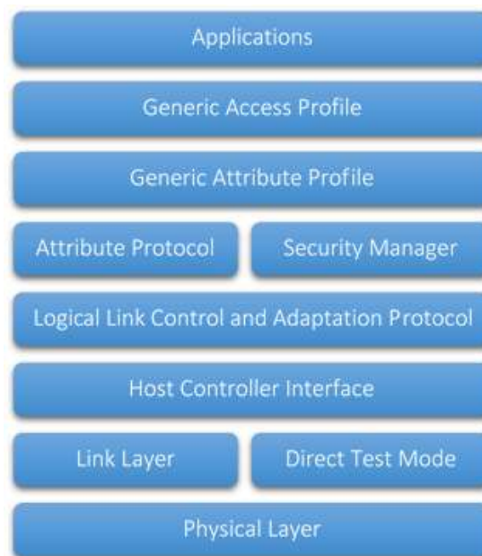
Figure 2.1: Block diagram picturing the Bluetooth smart stack
