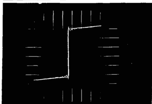
Figure 14.- AC Hysteresis Loop, Square Wave Excitation, 400, 800, 1600, and 3200 Hz, 0.004-Inch 4%Mo-79%Ni-17%Fe Toroid, Square Loop, 250° C
