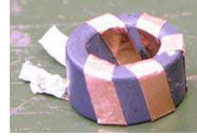
Fig. 3. An example of an inductor fabricated from copper foil and a commercial magnetic core.
