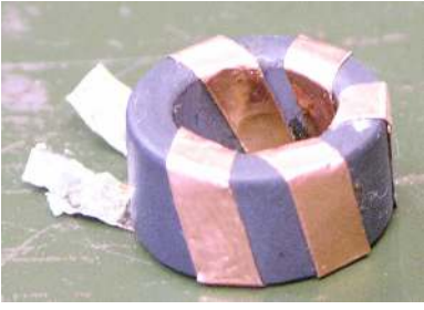
Fig. 3. An example of an inductor fabricated from copper foil and a commercial magnetic core.
