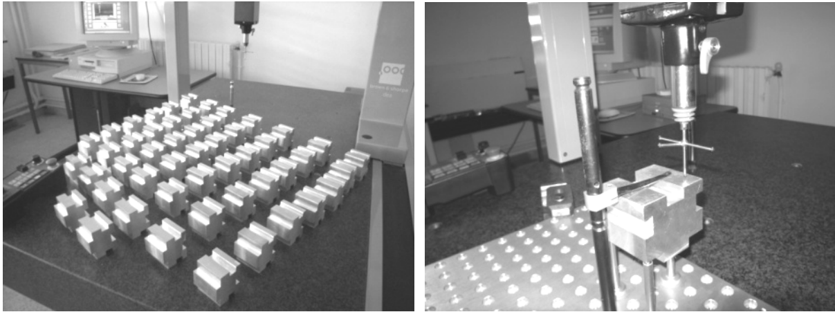
Figure 7: Final inspection on CMM.
