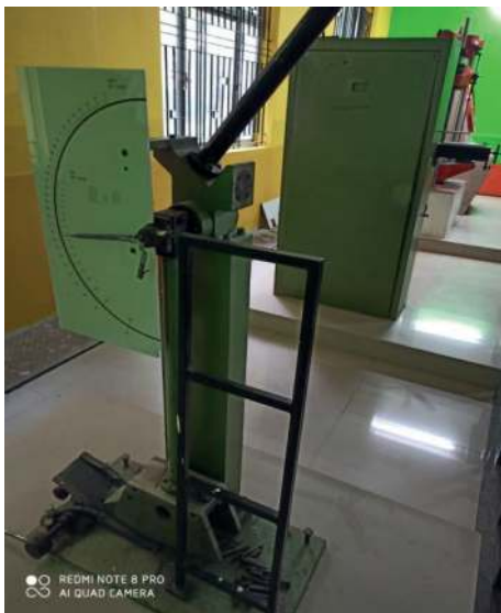
FIGURE 4: Impact test machine.
