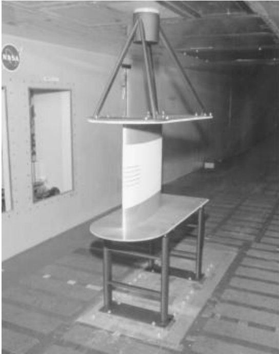
Figure 3. 53.3-cm-Chord NACA 0012 Model in IRT Test Section.
