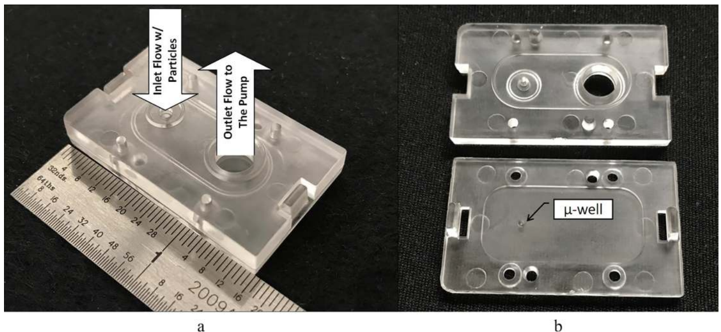
Fig 1. (a) The photograph of the assembled \mu -well aerosol collection cartridge and (b) the cartridge in a disassembled state.
