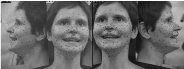
Figure 1: Gathering flashpoint positions using a photogrammetric method. Here 245 colored beads have been glued on the subject’s face.
