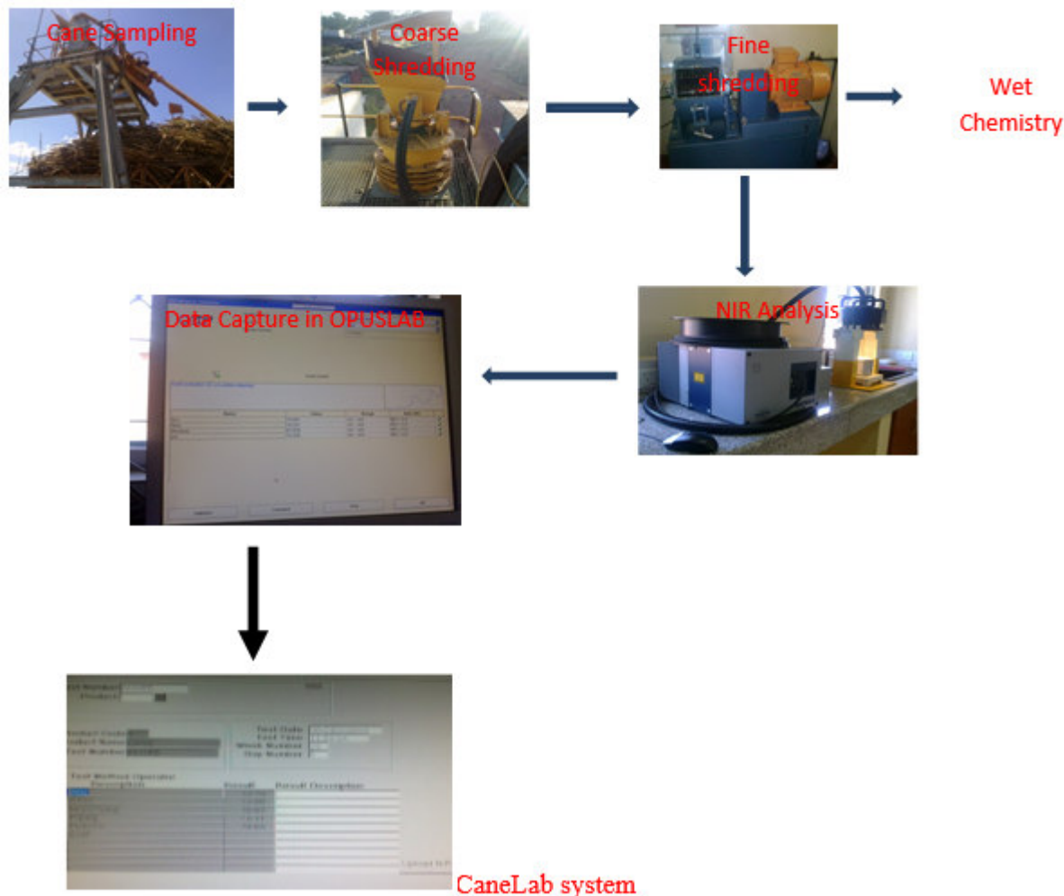
Figure 4: NIR analytical protocol for shredded cane at Nzoia Sugar Factory Pilot Cane Testing Unit.
