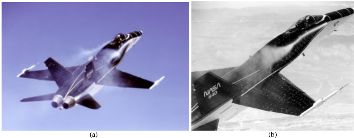
Figure 1. Flow Visualizations of Vortex from the LEX Bursting ahead of the Vertical Tail on an F/A-18 (Photographs Courtesy of the NASA Dryden Flight Research Center)
