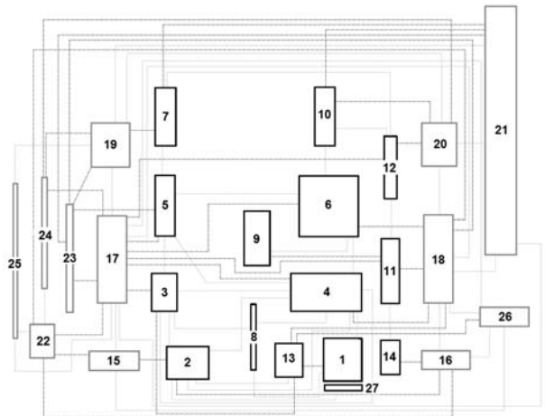
Fig. 11. Nodalization scheme of the EPR containment building.
