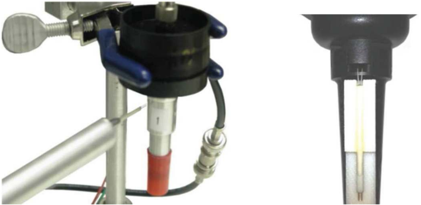
Figure 1. Hot-wire anemometer probes: placed near the inlet of a cyclone (left); held in a custom bracket and cemented onto a cyclone (right).
