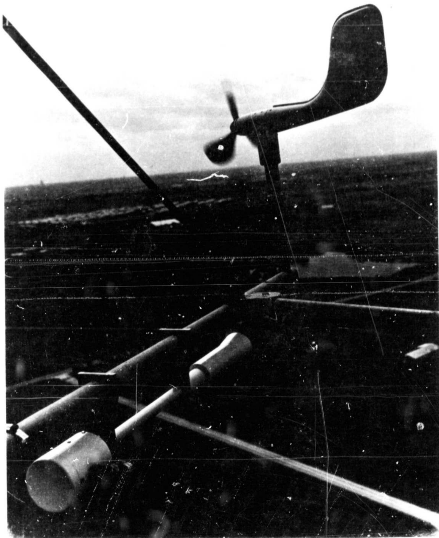
Figure 6. Aerovane wind transmitter and Climet aspirated radiation shield containing thermistor temperature sensor, mounted on tower instrument boom. View to southwest.
