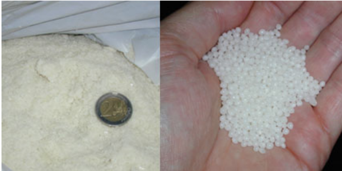
Figure 1. Sasobit® Flakes (Left) and Prills (Right).
