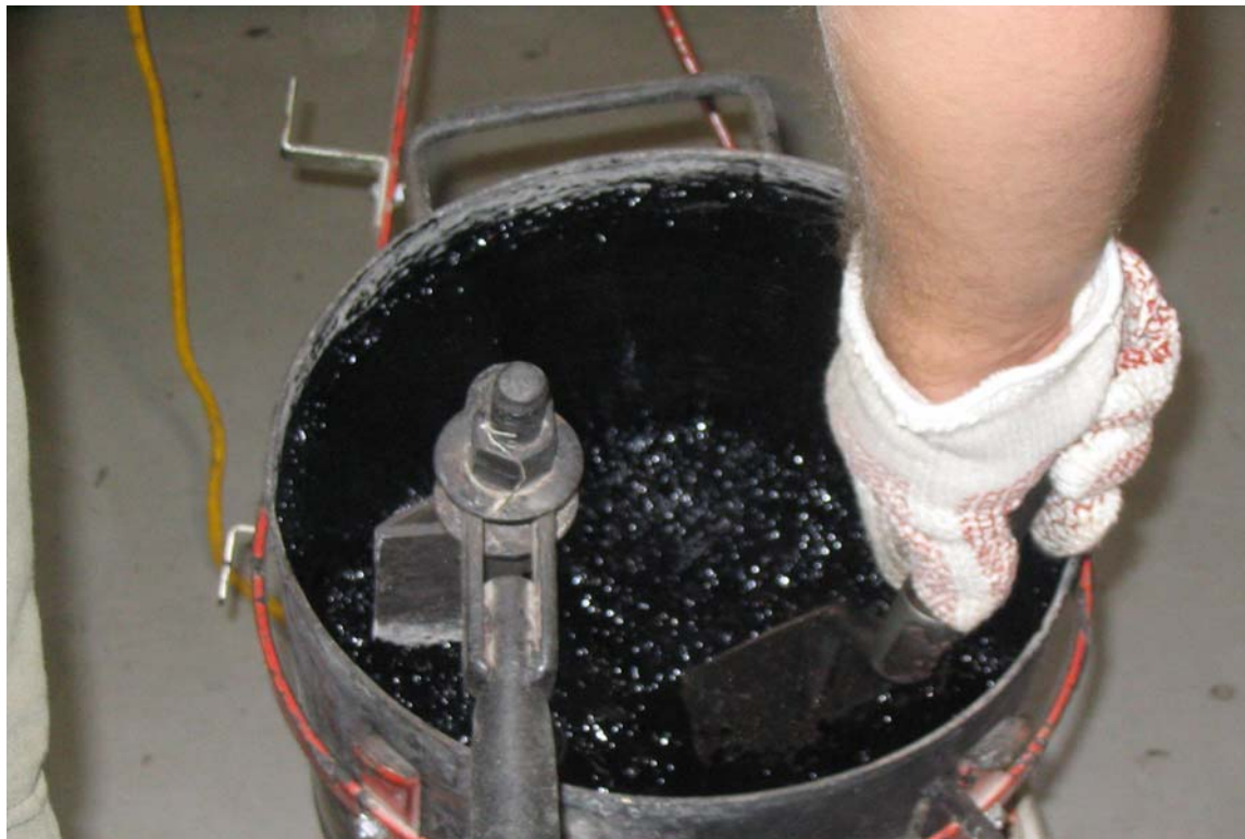
Figure 6. Hot Mix Asphalt in Bucket Mixer.
