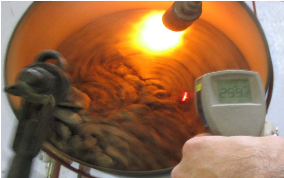
Figure 5. Heating of Wet Aggregate to Mixing Temperature.
