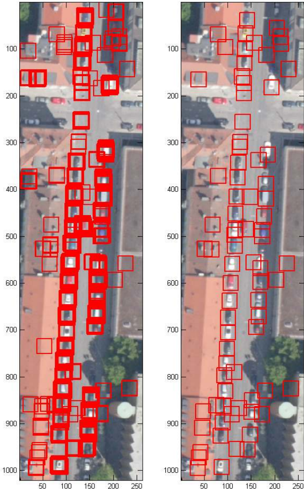
(a) without post-processing (b) with threshold and multi detection suppression
