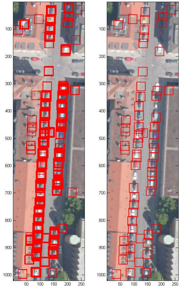
(a) without post-processing (b) with threshold and multi detection suppression
