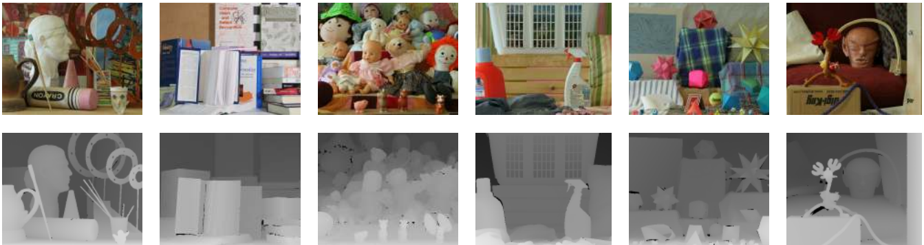
Fig. 3. The new Art, Books, Dolls, Laundry, Moebius, and Reindeer stereo pairs, which are used as test set.
