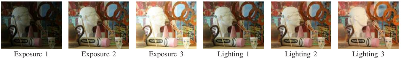
Fig. 12. The left image of the Art dataset with three different exposures and under three different light conditions. The right images have been captured under the same conditions, such that 3 \times 3 combinations of matching are possible, separately for different exposures and light conditions.
