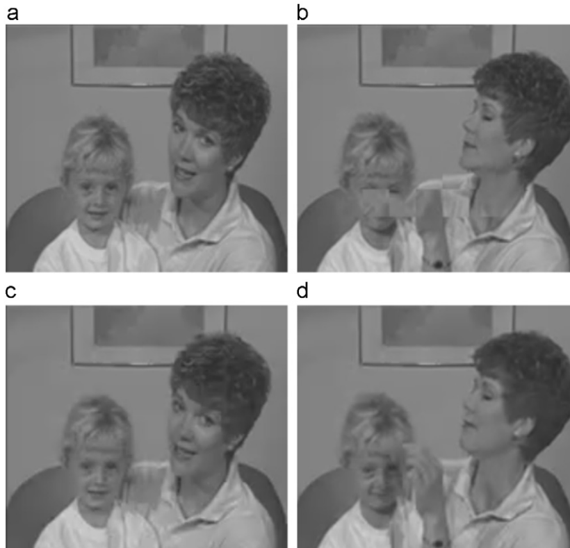
Fig. 9. (a) First frame in Case 2 (QP=24 without channel coding), PSNR=41.2 dB, SSIM=0.9765. (b) 16th frame in Case 2, PSNR=31.6 dB, SSIM=0.9125. (c) First frame in Case 3 (QP=30 with channel coding), PSNR=36.9 dB, SSIM=0.9443. (d) 16th frame in Case 3, PSNR=35.8 dB, SSIM=0.9326.
