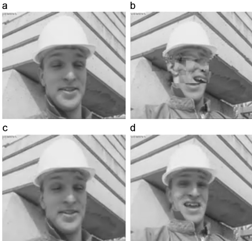
Fig. 6. (a) First frame in Case 2 (QP=24 without channel coding), PSNR=40.1 dB, SSIM=0.9731. (b) 35th frame in Case 2, PSNR=25.6 dB, SSIM=0.8497. (c) First frame in Case 3 (QP=30 with channel coding), PSNR=36.0 dB, SSIM=0.9489. (d) 35th frame in Case 3, PSNR=34.8 dB, SSIM=0.9369.
