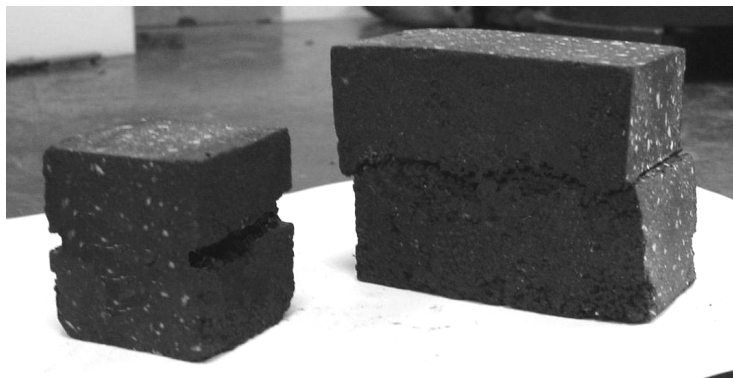
Figure 3: Specimens used in the mechanical tests carried out to evaluate the internal cohesion of the mastic
