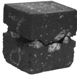
Figure 11: Failure zone usually observed in the specimens used in tensile tests
