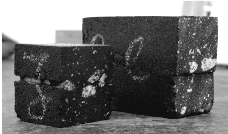
Figure 2: Specimens used to evaluate the strength of the bond between mastic and aggregates
