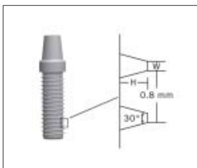
Fig 2 Schematic representation of the screw parameters: Zoom view of screw (right). H = height, W = width.
