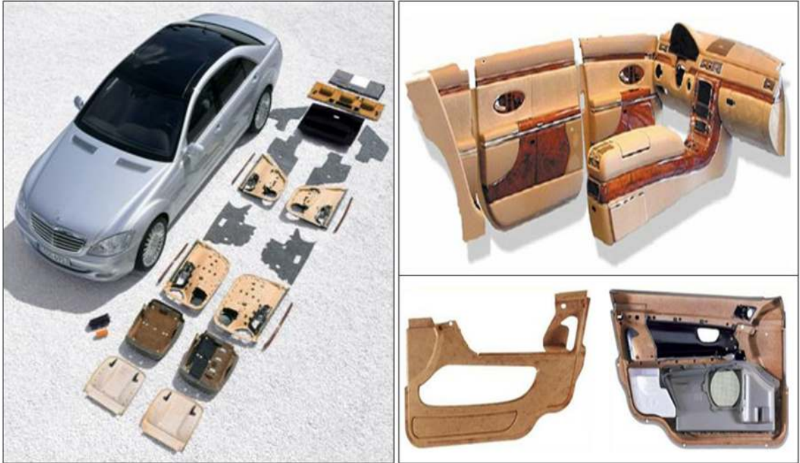
Figure 1. Automobile components based on polymer composites reinforced with lignocellulosic fibers.
