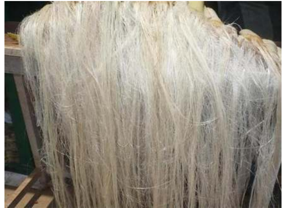
Figure 3. Pineapple fibers, PALF, extracted from the leaves of Ananas comosus .
