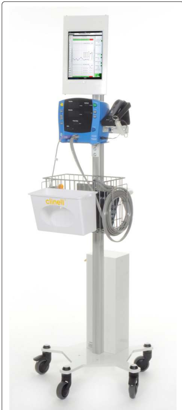
Fig. 1 The SEND data entry hardware. Observation roll stand with equipment for taking observations, barcode scanner and tablet computer
