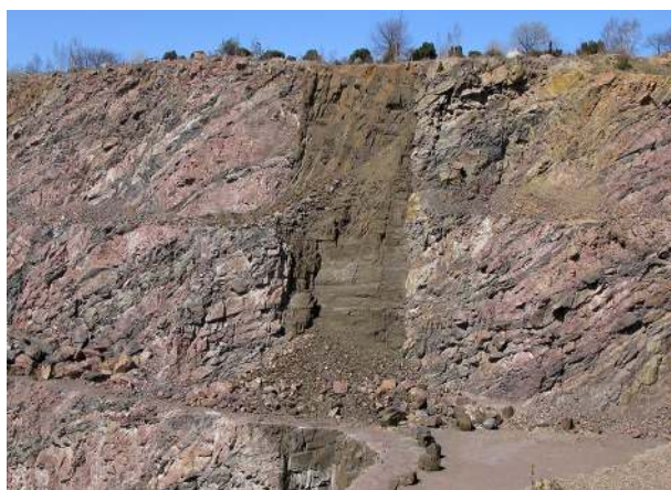
Fig. 3 Photo from Dalby quarry exemplifying the rock mass composition with severely fractured reddish gneiss and numerous variably thick dykes and schlieren of metabasite. The photo also shows a subvertical brownish black Permo-Carboniferous dolerite dyke cutting through the host rock. Photo: L. Johansson
